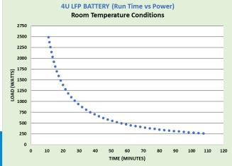
LFP inherent qualities such as chemical stability and low resistance provide the best chemistry to deploy for uninterruptible power supplies. In addition to improved performance, Acumentrics' LFP Battery Packs provide safety protection at three levels: system, pack and chemistry.
