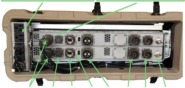
Critical N+1 SNMP RS232 DC DC AC Ground AC Outputs\*\* Conn\*\* Comm. Comm. Output\*\* Input\*\* Input\*\* Pin Note\*\*: connectors on each UPS, copper alloy contacts with gold plating; [50µm Au plating thickness]:
