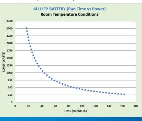
LFP inherent qualities such as chemical stability and low resistance provide the best chemistry to deploy for uninterruptible power supplies. In addition to improved performance, Acumentrics' increased runtime LFP Battery Packs provide safety protection at three levels: system, pack, and chemistry
